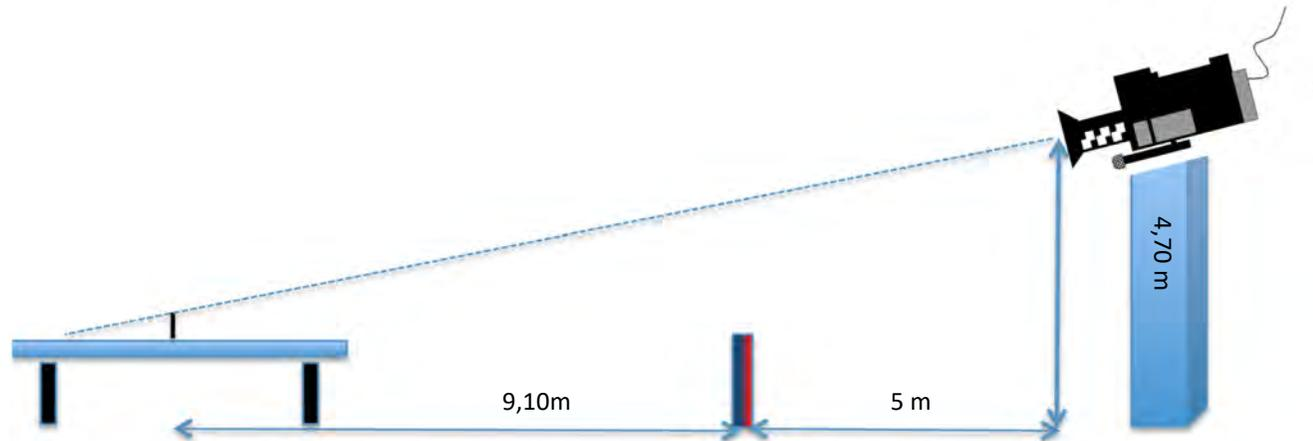
**REFERENCE : Height of the main camera to provide with the right shot angle**
