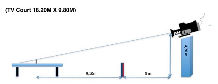
**REFERENCE : Height of the main camera to provide with the right shot angle** 5 m behind the line of surrounds = 14,10m from the middle of the table Main camera should be at 4,70m
