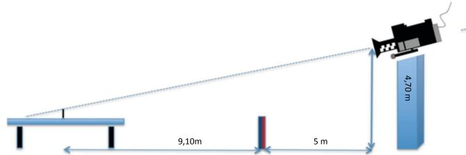
REFERENCE: Height of the main camera to provide with the right shot angle 5 m behind the line of surrounds = 14,10m from the middle of the table Main camera should be at 4,70m
